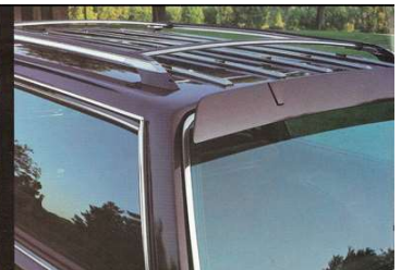
The available tailgate air deflector directs wind across the rear window to help keep dirt and debris off the glass.
